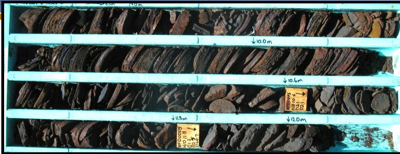
Regolith goethite “biscuity” ore > 40% Fe (above) Shows iron flooding on cleavage planes
